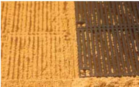
GRATE embedding with concrete sand, geogrid profile remains after GRATE removal
